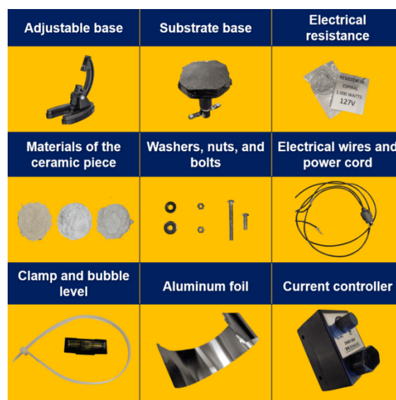
Figure 2. Materials that integrate the wettability device.
