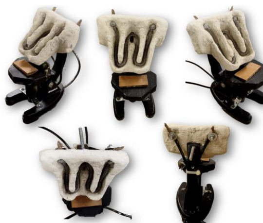
Figure 7. Display of the developed wettability device (without aluminum sheet) from various perspectives.
