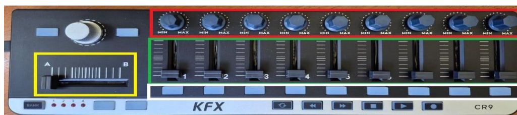
Figure 2. The CR-9 (KFX, China) MIDI controller used for the desired performance (Source: authors).
