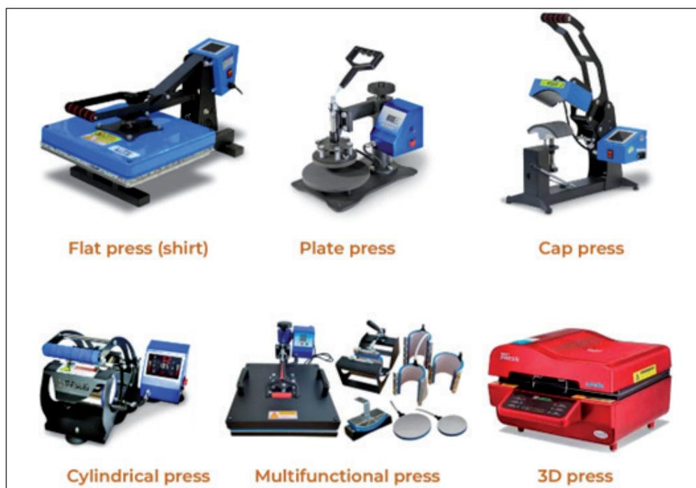
Figure 5: Examples of described press types used in sublimation.
